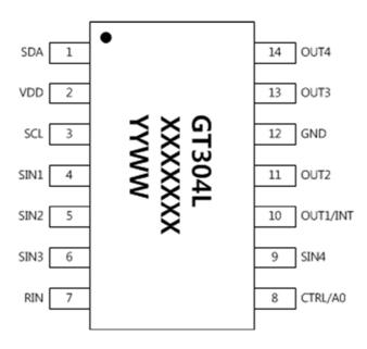
Figure 4.1 SOP14L Pinout Diagram (Top View)
