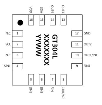
Figure 4.2 QFN16L Pinout Diagram (Top View)
